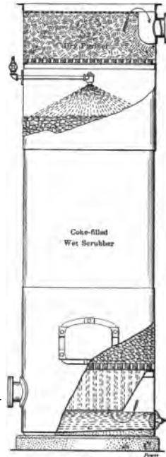
FIG. 90.—Combined Wet and Dry Scrubber.
